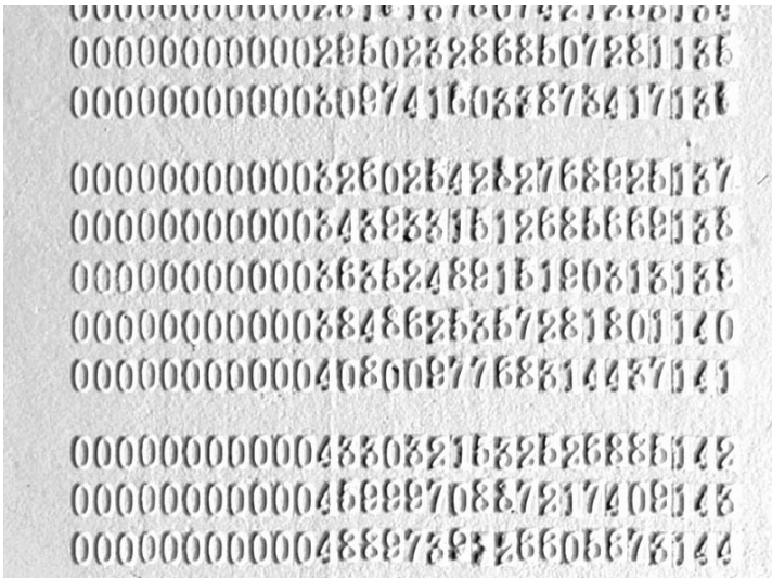
Figure 8. Experimental stereotype mold in plaster of paris. Detail. (Photo courtesy of the Science Museum, London.)
